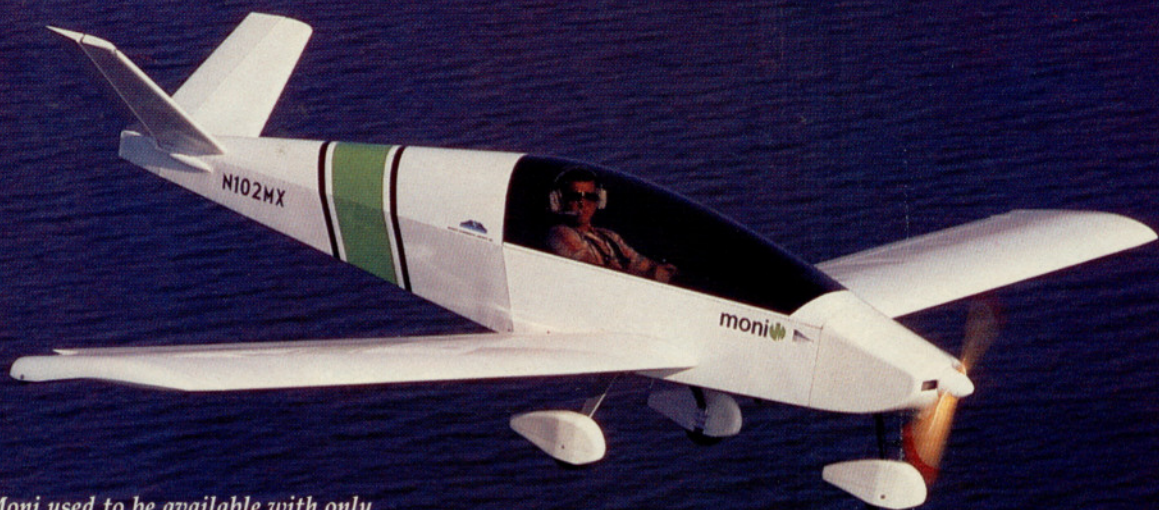
The Inav Moni used to be available with only one wheel, a la sailplanes. The new tricycle gear option simplifies ground operations.
